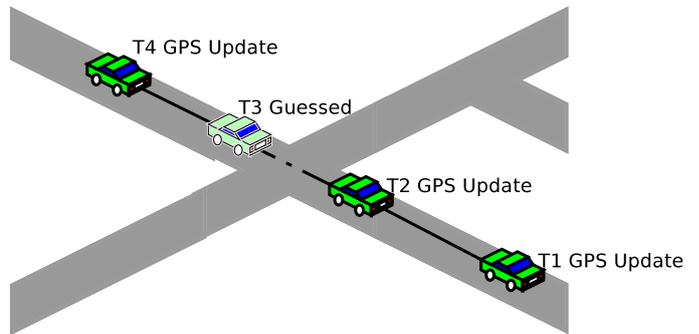
Fig. 1: Estimated position system example.
