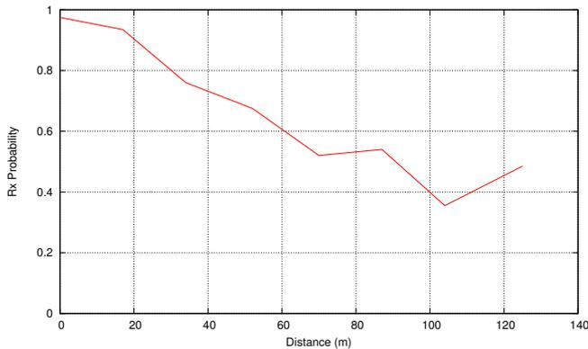
Fig. 3: LOS Rx Probability vs Distance.
