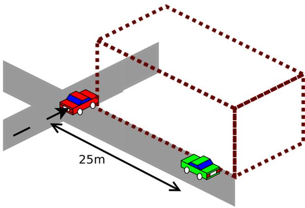
Fig. 4: Location of the cars for NLOS measuring.
