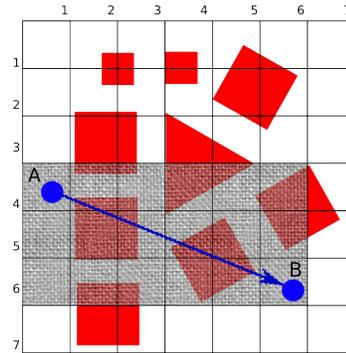
Fig. 2: For each source-destination pair, the model only iterates over obstacles inside the rectangle defined by locations  $A$  and  $B$ .
