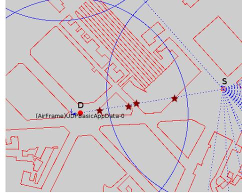
Fig. 1: Screenshot from the VEINS simulator. Stars represent the intersection of the transmission line with the obstacles' walls.
