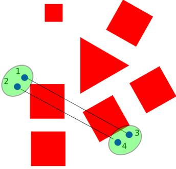
Fig. 3: A transmission from node 1 to node 3 will experience the same attenuation than a transmission from node 2 to node 4.
